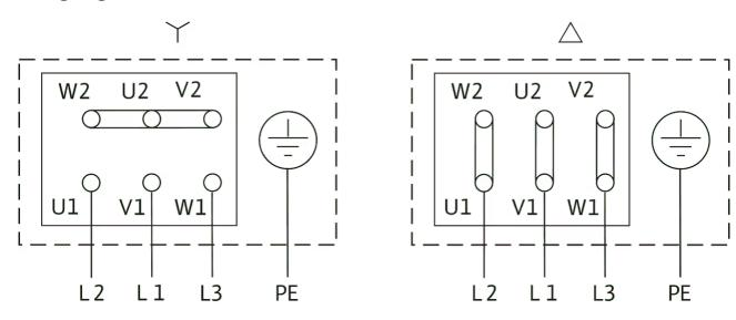
$\Delta\text{:}$  Connection diagram delta connection
