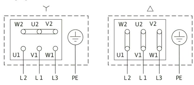
$\Delta\text{:}$  Connection diagram delta connection
