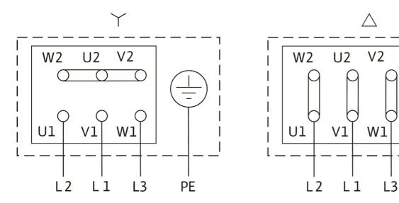
$\Delta\text{:}$  Connection diagram delta connection
