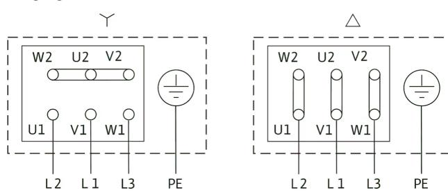
$\Delta\text{:}$  Connection diagram delta connection
