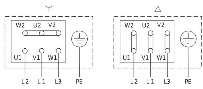
$\Delta\text{:}$  Connection diagram delta connection
