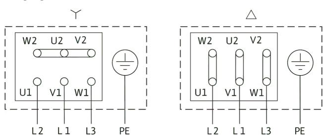
$\Delta\text{:}$  Connection diagram delta connection
