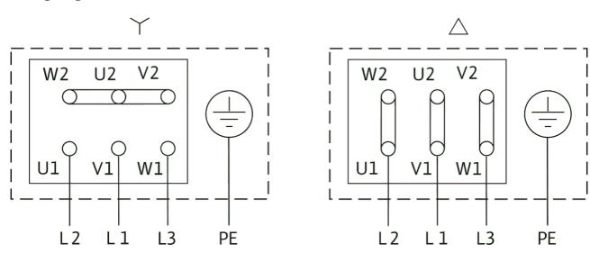
$\Delta\text{:}$  Connection diagram delta connection
