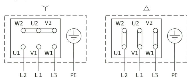
$\Delta\text{:}$  Connection diagram delta connection
