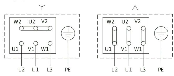
$\Delta\text{:}$  Connection diagram delta connection
