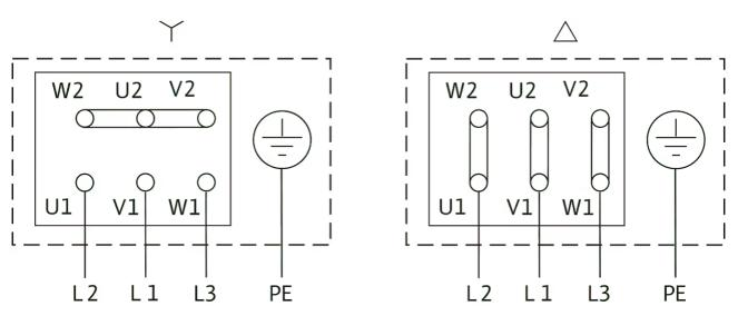
$\Delta$ : Connection diagram delta connection
