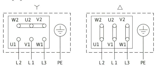
$\Delta\text{:}$  Connection diagram delta connection
