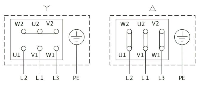
$\Delta$ : Connection diagram delta connection
