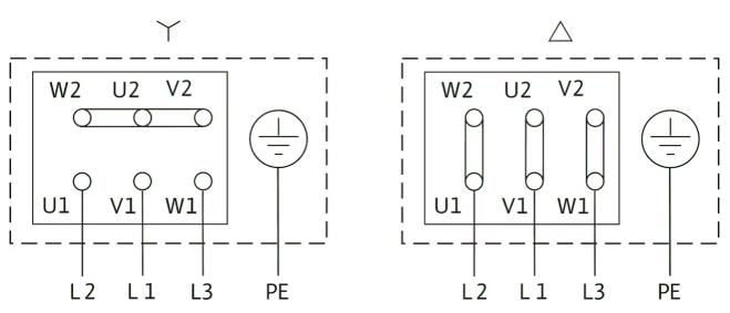
$\Delta$ : Connection diagram delta connection
