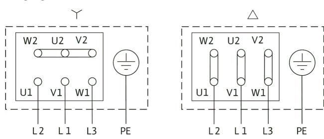
$\Delta\text{:}$  Connection diagram delta connection
