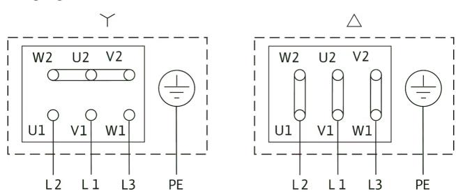
$\Delta\text{:}$  Connection diagram delta connection
